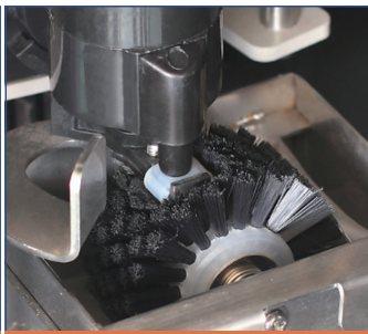
Rolling brush help to clean nozzles
