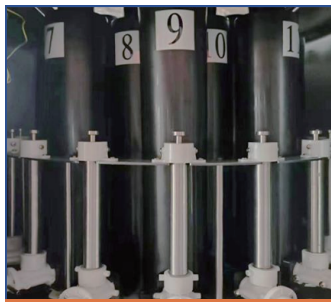
Colorant Recirculation Nozzle Design
